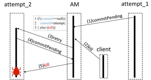
Fig. 13. MR-5009 detected by CLOUDRAID with log enhancement.
