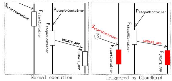
Fig. 11. A new atomicity violation detected by CLOUDRAID. The messages and their handlers triggering the bug are highlighted in red.
